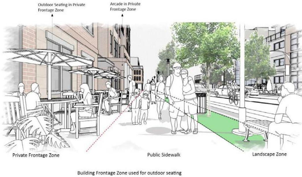
Figure V-8: Examples of Building Frontage Zone Activity
