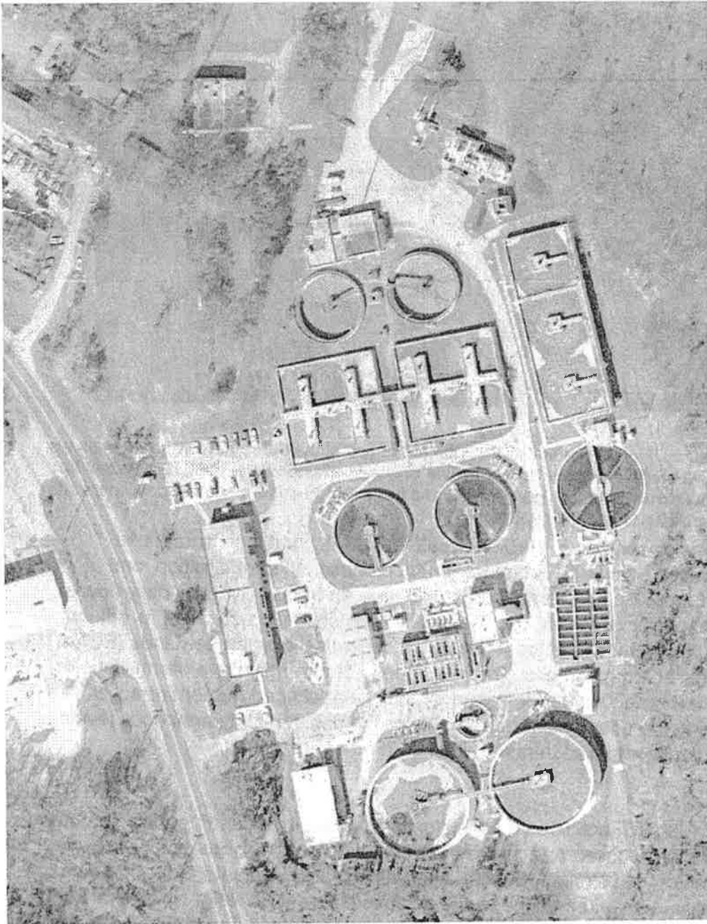
FIGURE 6 Main Street Water Reclamation Facility Aerial Photograph Illustrating Two Parallel Advanced Secondary Treatment Trains. Final Chlorine Contact Chamber for Disinfection is on the Lower Right of the Photo and is the Last Point in the Process before Discharge to Sweetwater Branch.
