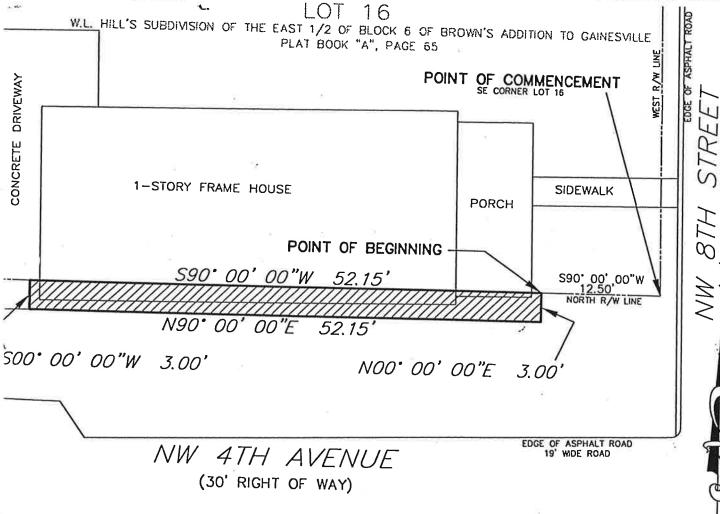
Bearings shown hereon are referenced to north right of way line of Northwest Fourth Avenue as bearing \$90' 00' 00"W.
