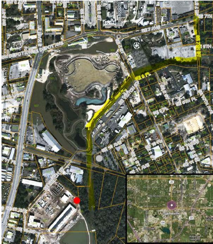
Figure 3-9. Proposed Natural Gas Pipeline and Facility Location.
