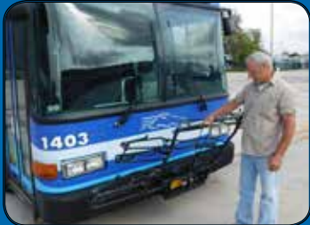
1. Pull up on release and lower rack.
