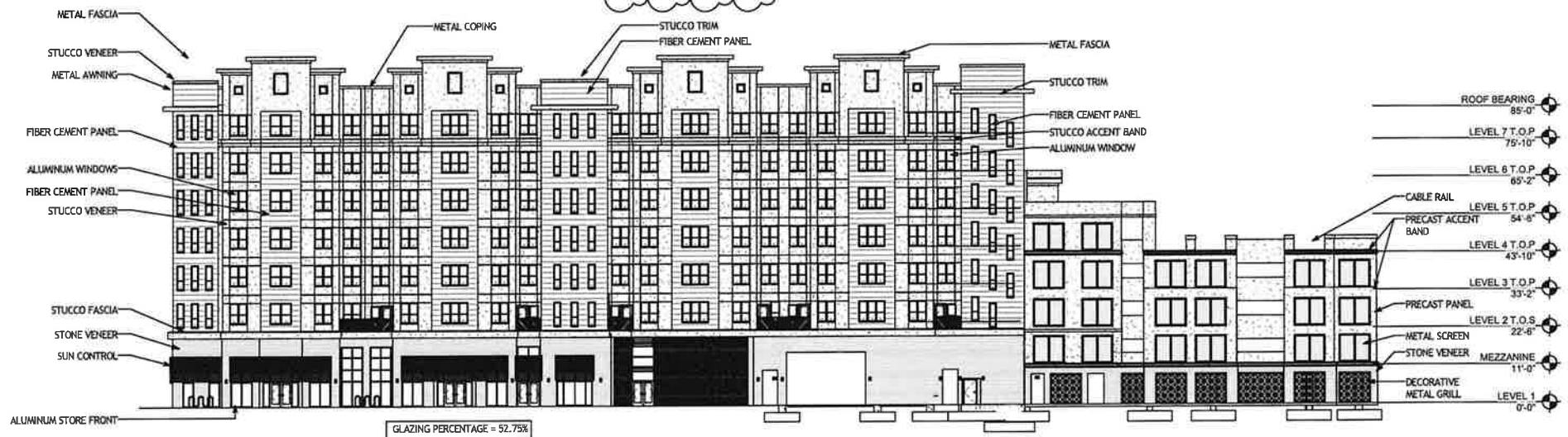
1 ELEVATION- EXTERIOR- SOUTH A3.01 1/16" = 1'-0"
