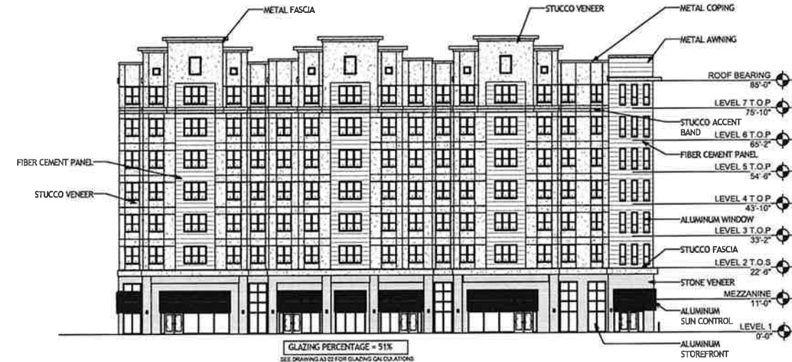
2 ELEVATION- EXTERIOR- WEST A3.00 1/16" = 1'-0"
