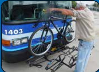
2. Place bike wheels into slots labeled “front” and “rear.” Pull out bike support and lift it over front wheel. The spring in the arm will keep your bike secure while the bus is moving.
