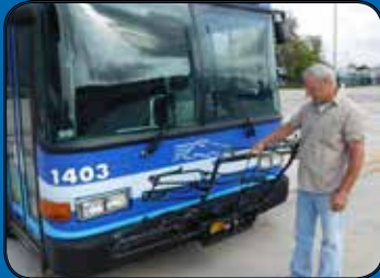
1. Pull up on release and lower rack.
