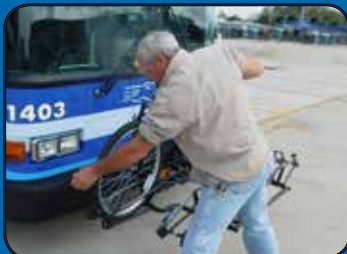
3. To unload, release support arm and lift bike from the rack. Return rack to the upright position.
