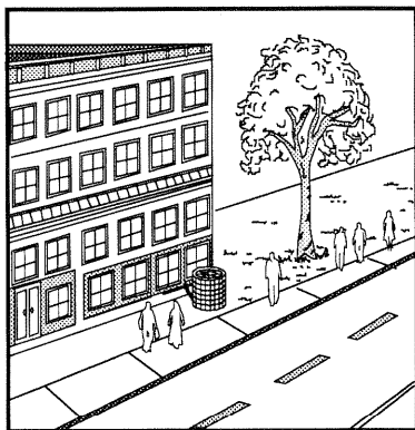
#19 Inappropriate front location for mechanical equipment
