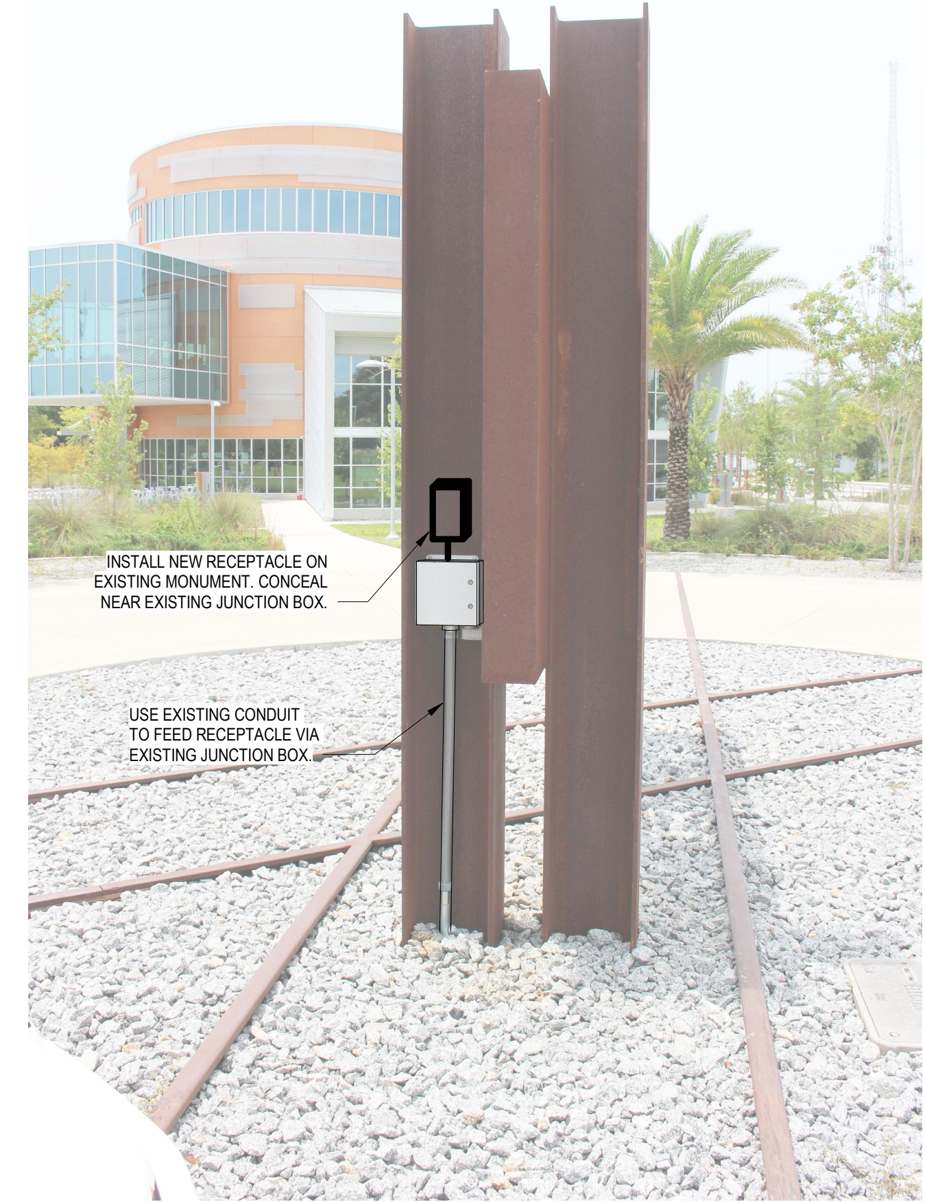
1 MONUMENT RECEPTACLE MOUNTING DETAIL NOT TO SCALE
