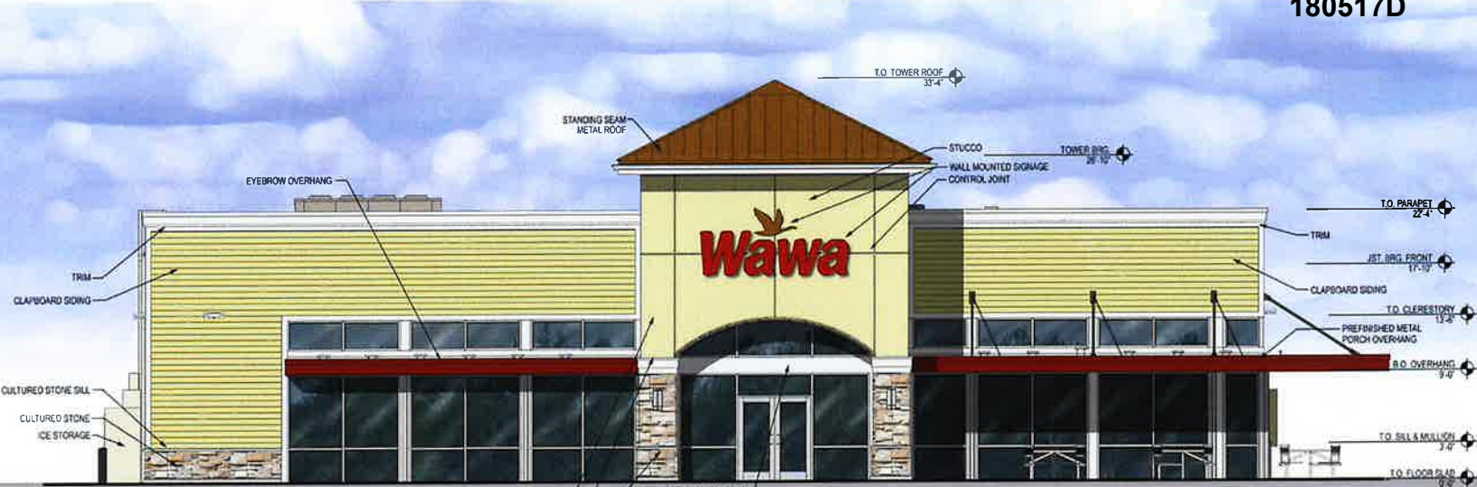
FRONT (EAST) ELEVATION (SE 11TH ST.) 68% WINDOW GLAZING BETWEEN 3'-0" AND 8'-0" A.F.F.
