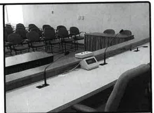
Pictured above is a typical queuing/voting system with queuing stations and the chairperson's LCD display.
