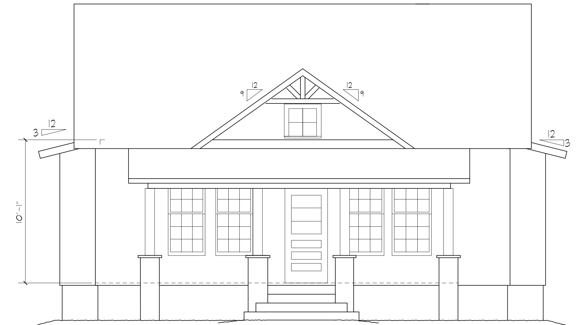
PROPOSED FRONT ELEVATION SCALE 1/4" = 1.0'
