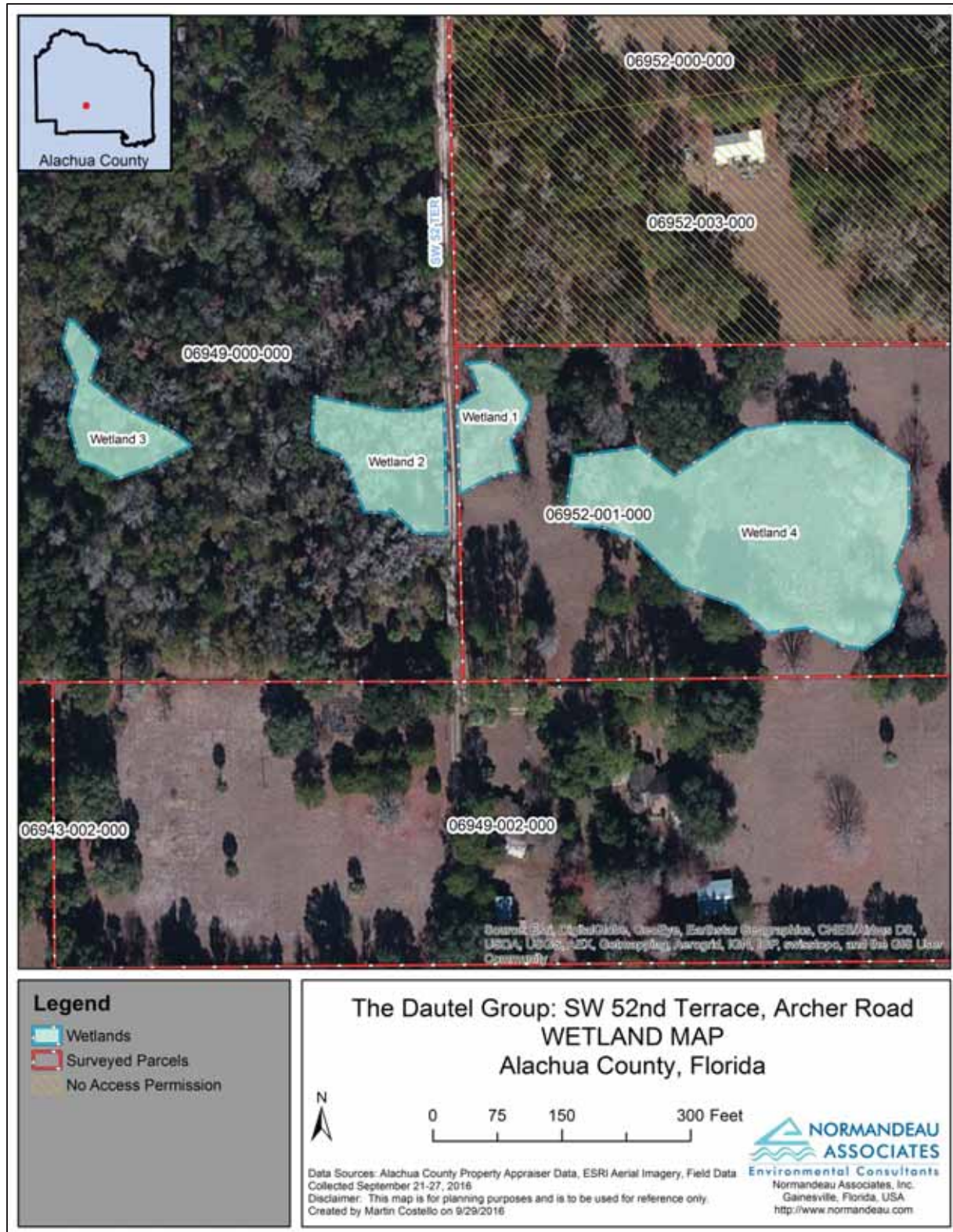
Figure 10. Wetlands delineated within the project boundary.
