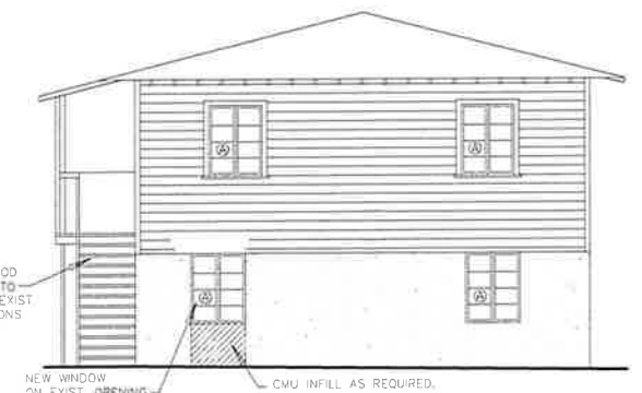
PROPOSED WEST ELEVATION N.T.S.
