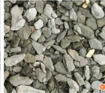
1 compacted crushed slate 5/8" minus size
