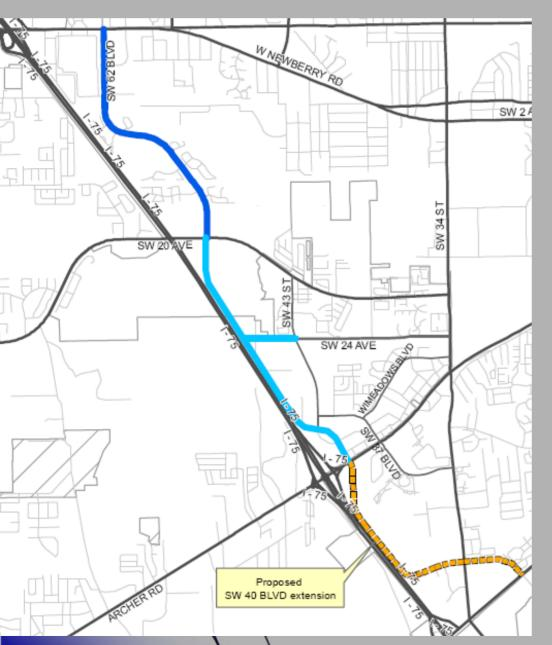
Proposed: Extension of SW 62nd Blvd / SW 52nd St as a new 4-lane segment south of SW 20th Ave, connecting to Archer Rd at SW 40th Blvd; also includes the extension of SW 24th Ave from SW 43rd St west to SW 62nd Blvd
