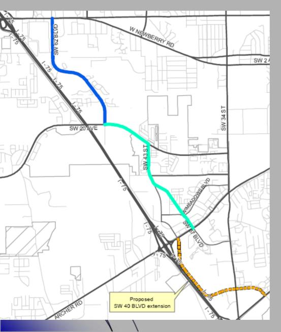
Proposed: 4-laning of existing roadways: SW 20th Ave between SW 62nd Blvd and SW 43rd St; SW 43rd St south to SW 24th Ave; new roadway alignment connecting to Archer Rd at SW 37th Blvd
