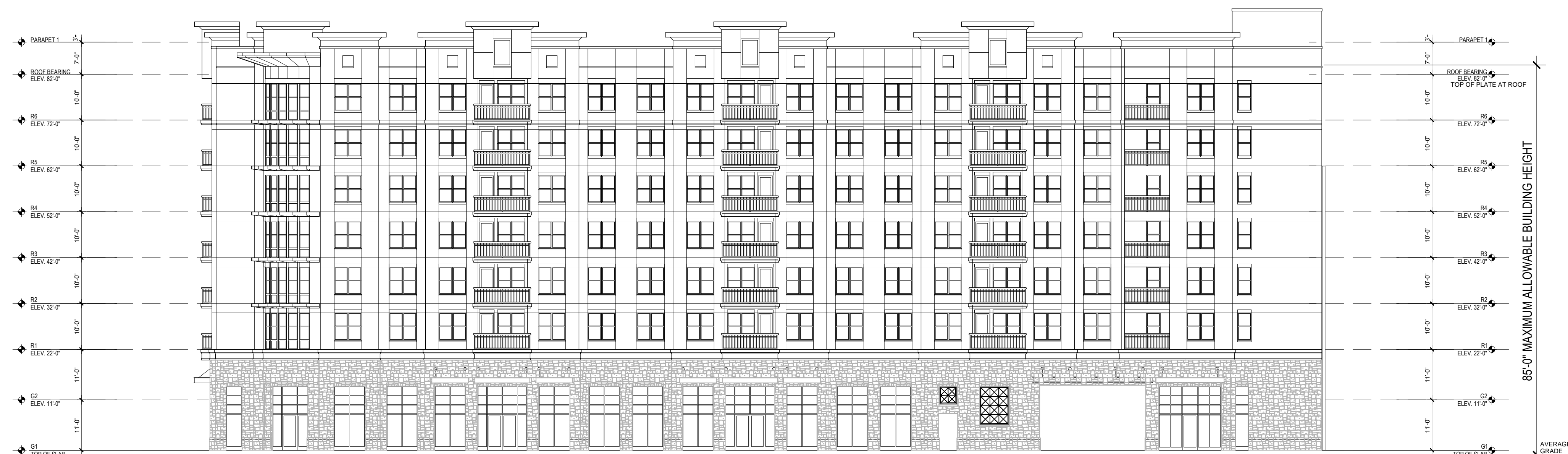
ELEVATION 1 SOUTH ELEVATION 1/16" = 1'-0" A4.00
