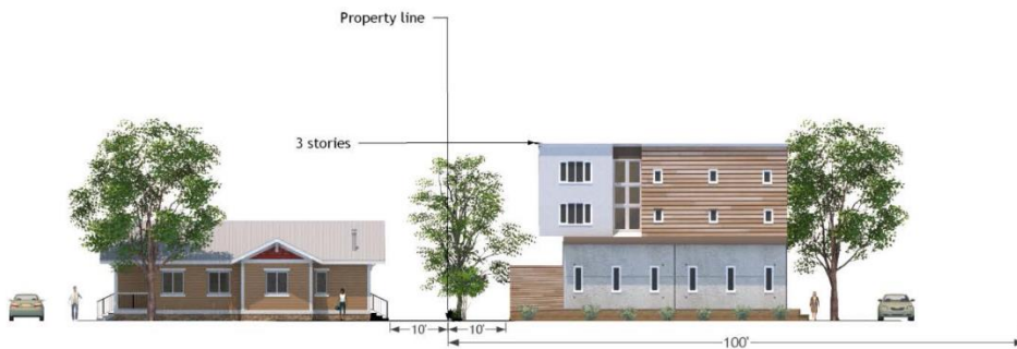
Figure 2: Height Compatibility Flat Roof Example
