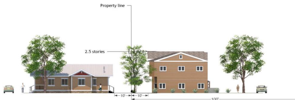
Figure 1: Height Compatibility Pitched Roof Example
