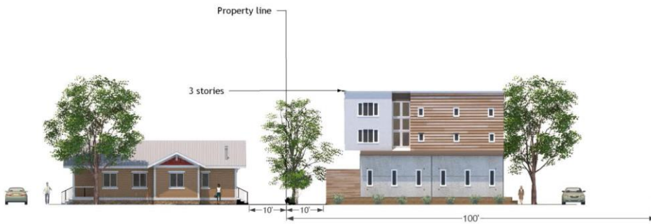
Figure 2: Height Compatibility Flat Roof Example
