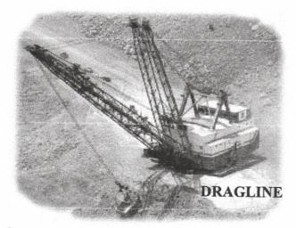
A dragline (which can weigh up to 8 million pounds with a base as big as a gymnasium and as tall as a 20-story building) digs into rock to expose the coal. It moves 100 or more cubic yards in a single bite--each cubic yard can fill the back of a half-ton pickup truck. Exposives and massive machines allow coal companies to hire fewer workers. A small crew can tear apart a mountain.
