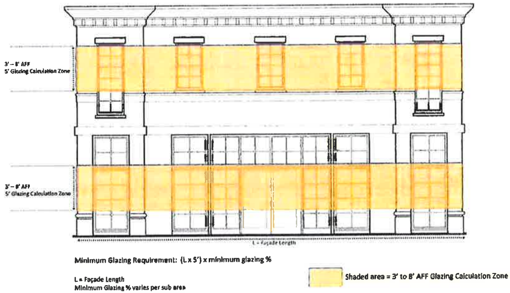
Figure 8: Glazing Requirements Diagram
