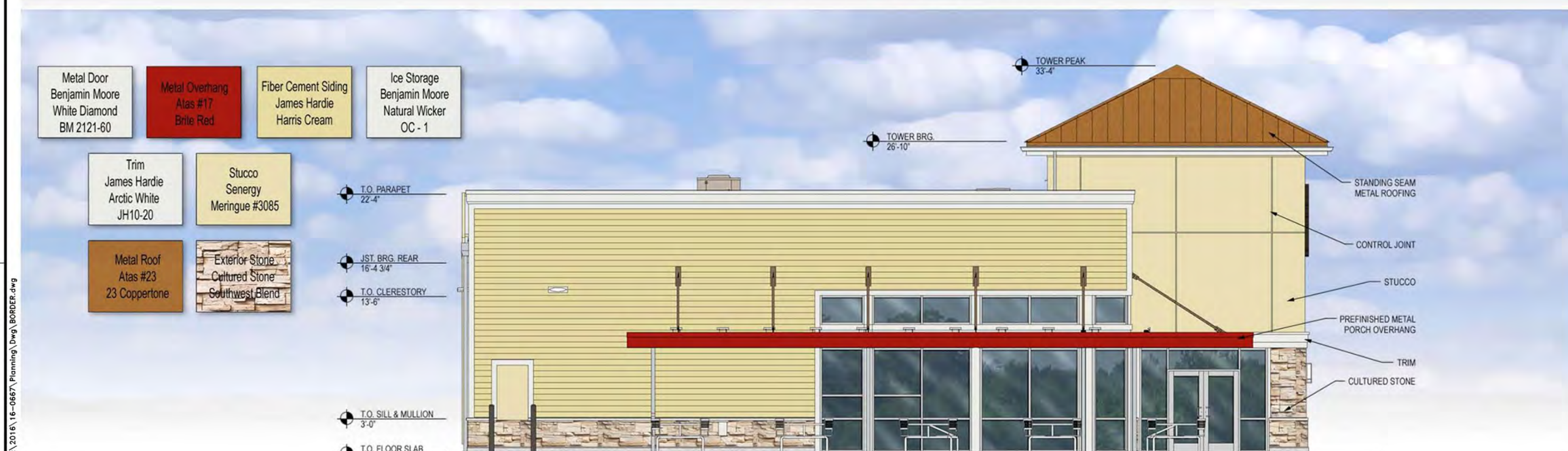
LEFT (NORTHWEST) ELEVATION (SW ARCHER RD.) 44% WINDOW GLAZING BETWEEN 3'-0" AND 8'-0" A.F.F.
