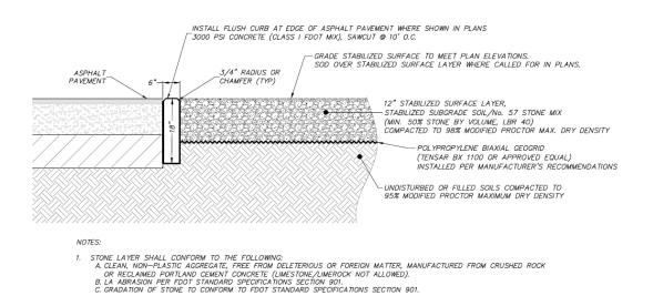
Ribbon Curb shall be provided at the edge of asphalt pavement when adjacent to the Stabilized Path. The curb and path location is shown on sheets 17, 18, 19, and 20
