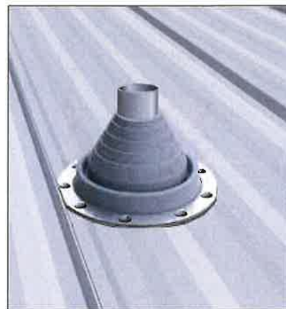
Fig. 13 Pipe Boots provide a water-tight seal around roof vents and come in a variety of sizes. They seal with caulk under the base and around the pipe. To assure water tightness of the roof, avoid installing over panel ribs.
