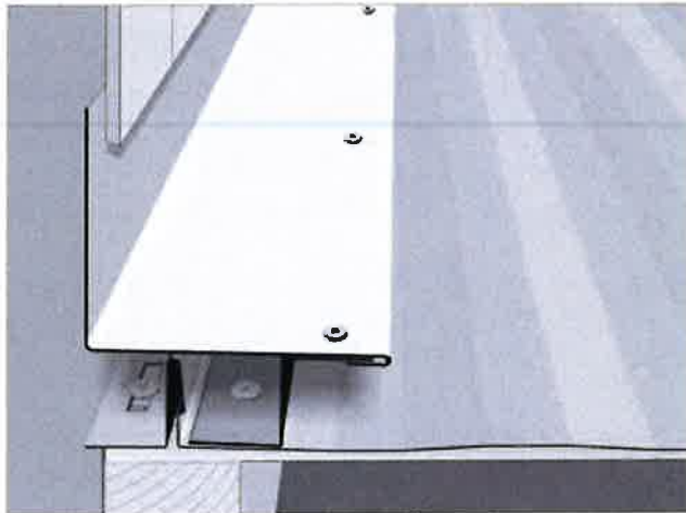
Fig. 17 Standard SW-7 Sidewall attaches to z-flashing with rivets and is covered on the wall side by siding.
