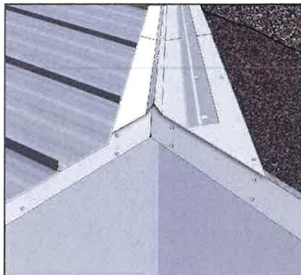
Fig. 19 Diagonally-cut panels are hemmed and attached to panel starter that is mounted on the surface of the valley.
