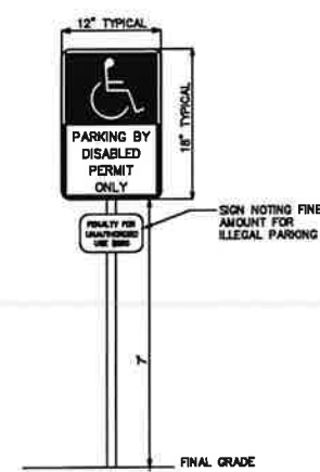
SIGN NOTES: 1. SIGN TO BE MADE OF 0.063" STEEL PAINTED WITH TRAFFIC PAINT 2. HANDICAP SIGN TO BE AS SHOWN ABOVE OR AS REQUIRED BY LOCAL CODE PAINT SIGN BLUE AND WHITE HANDICAP PARKING SIGN DETAIL N.T.S.
