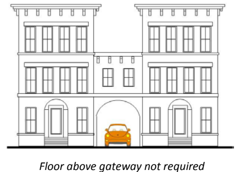
Figure V - 4: Example of Gateway
