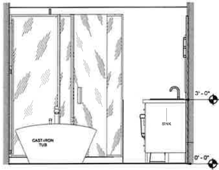
BATHROOM - WEST INTERIOR ELEVATION SCALE: 1/2" = 1'-0"
