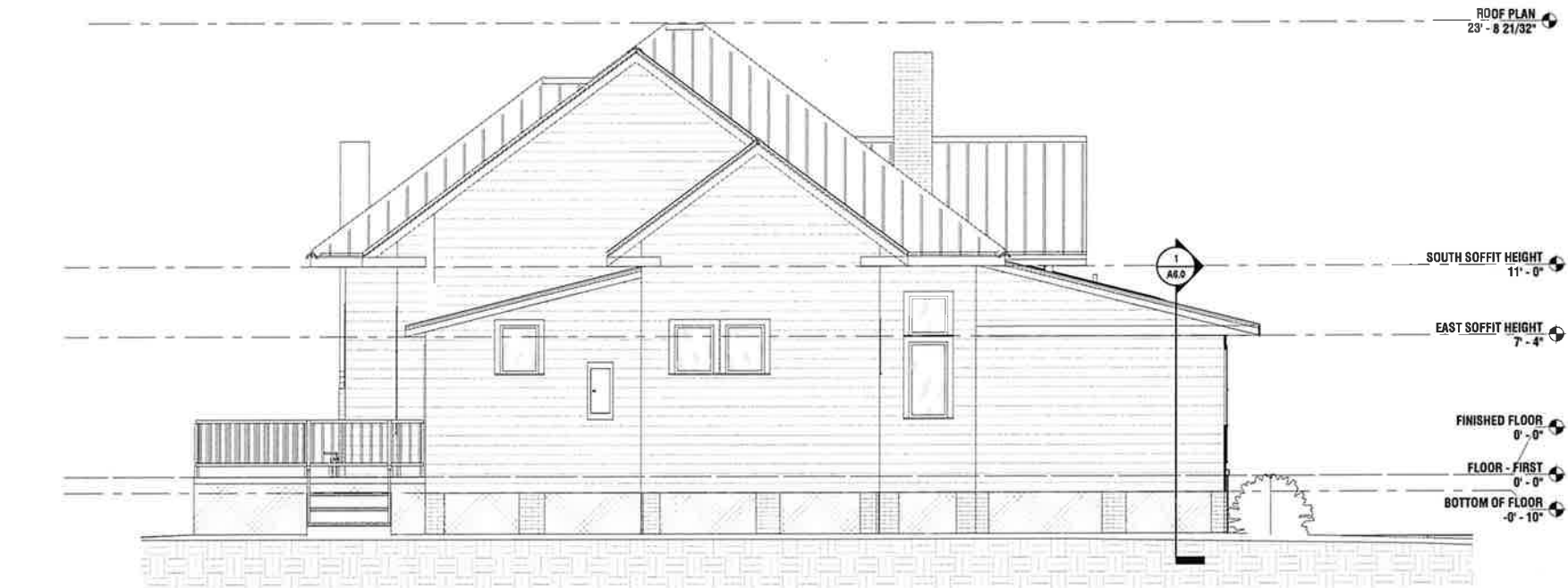
SOUTH ELEVATION SCALE: 1/4" = 1'-0"
