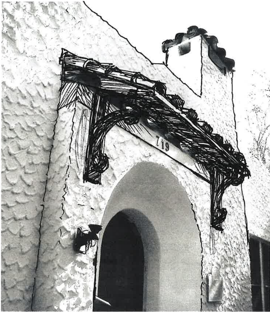
Proposed view of extended tile roof over entry supported on new steel brackets. Tile work on chimney top will be restored. Building exteriors will be completely repainted and all screens restored.
