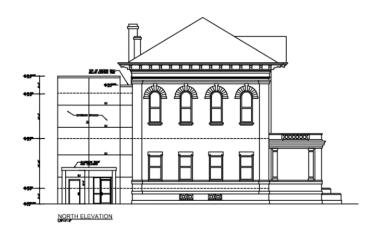
There is also a new addition proposed. The two story addition will be located to the rear along NE 3<sup>rd</sup> Avenue. The addition will be masonry and stucco and used to house the elevator, fire rated exit stairs and two handicap restrooms on both floors. The mechanical equipment will be mounted on the roof and concealed with a parapet wall. A new exterior exit and covered landing is proposed on the east elevation.
