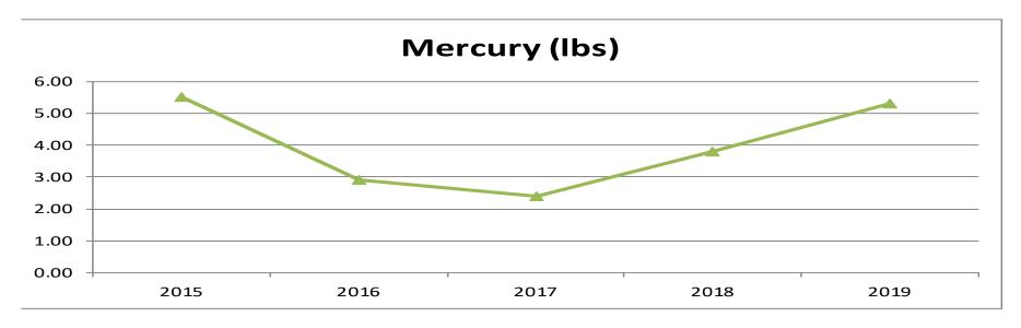
Mercury was lower in 2016 and 2017 due to higher removal rate settings to assure compliance with the MATS Rule.
