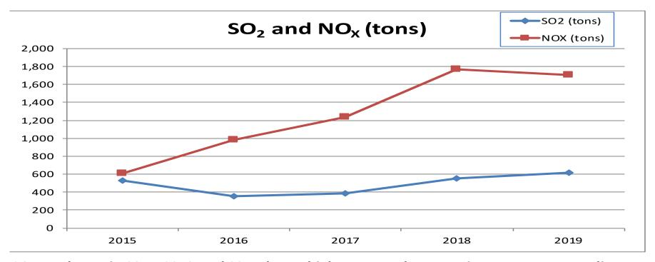
${\rm SO_2}$  was lower in 2015, 2016, and 2017 due to higher removal rate settings to assure compliance with the MATS Rule.
