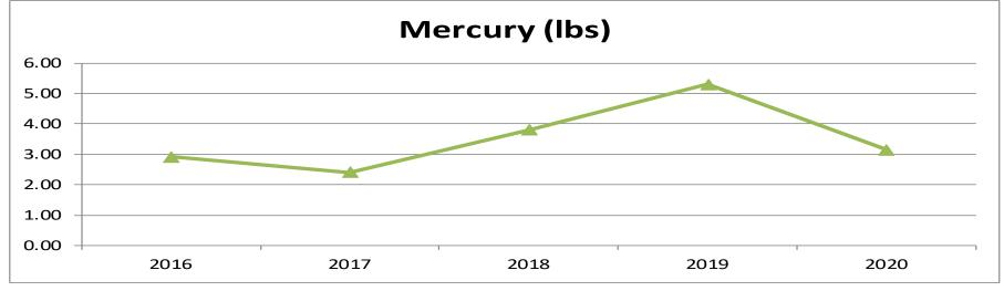
Mercury was lower in 2016 and 2017 due to higher removal rate settings to assure compliance with the MATS Rule.
