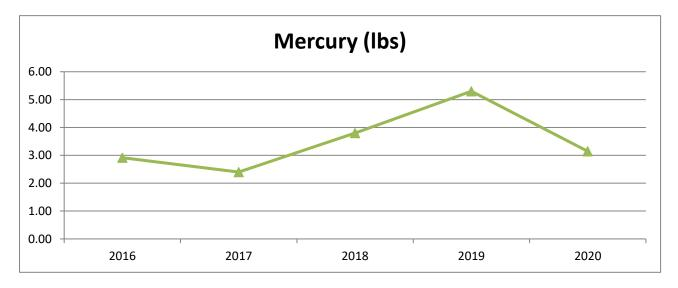
Mercury was lower in 2016 and 2017 due to higher removal rate settings to assure compliance with the with the MATS Rule.
