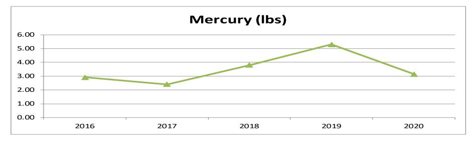
Mercury was lower in 2016 and 2017 due to higher removal rate settings to assure compliance with with the MATS Rule.
